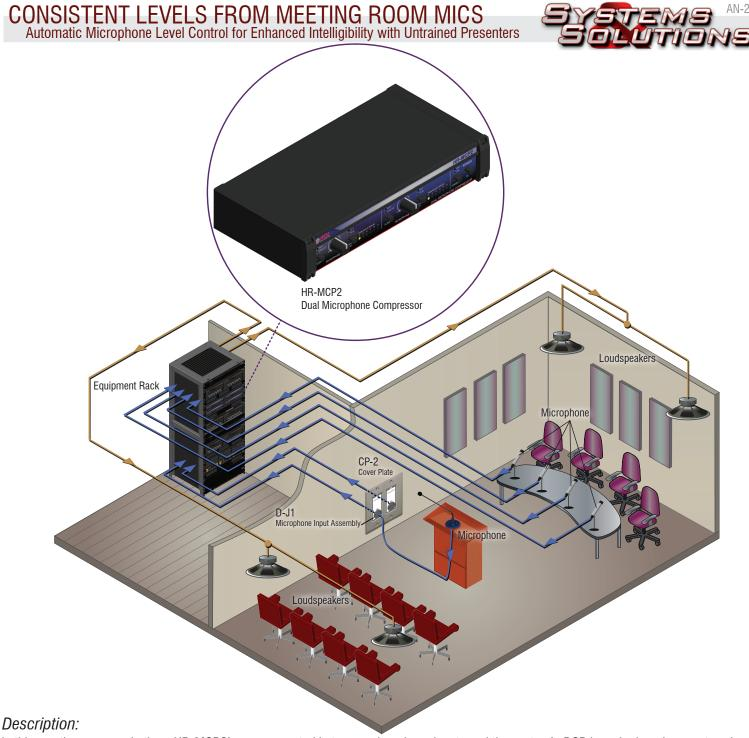
In this meeting room rack, three HR-MCP2's are connected between microphone inputs and the system's DSP based microphone auto-mixer to reduce demands on the DSP's resources while providing consistent levels from each of the system's six microphone inputs. The HR-MCP2 improves sound quality and intelligibility by producing consistent audio levels and controlling overloads that produce distortion and clipping at the DSP inputs.
