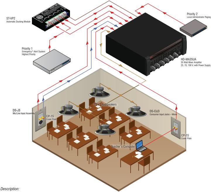
Classroom mic, line and computer audio sources are connected to the HD-MA35UA Mixer Amplifier through RDL wall plates. A school-wide paging feed connects directly to the mixer amplifier paging input. The paging source may be either mic or line level. VOX switching eliminates the need for push-to-talk contacts. The HD-MA35UA setup allows flexibility in muting or ducking the other input channels during paging.
