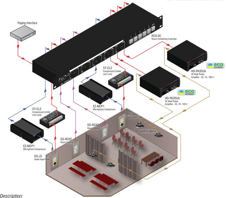
This cafetorium can be used as one large room or as two smaller rooms formed by movable wall partitions. Each room has one mic and one mono or stereo line-level input connection through a DS-J3 input plate. EZ-MCP1 Microphone Compressors provide consistent level and overload protection on the mic inputs. ST-CL2 Compressor/Limiters provide the same benefits for the line inputs.
