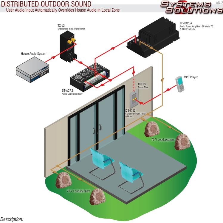
An unbalanced stereo audio signal from the house audio system is summed and converted to a balanced mono signal using the TX-J2 Unbalanced Input Transformer. The ST-ACR Audio Controlled Relay normally connects the house audio source to the FP-PA20A 20 Watt Audio Power Amplifier which feeds 70 Volt outdoor loudspeakers in the patio seating area.
