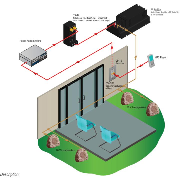
A stereo unbalanced audio signal from the house audio system is summed and converted to a balanced mono signal using the TX-J2 Unbalanced Input Transformer. The patio is equipped with a DS-CIJ3 Consumer Input Jack Decora® plate that provides connectivity for an MP3 music player or other stereo audio source. Source selection is controlled by the house audio system and volume is controlled using the house audio system and/or the MP3 player, if it's in use.
