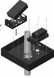
2. Secure the tray by tightening the hose clamp to mounting brackets using a screwdriver.
