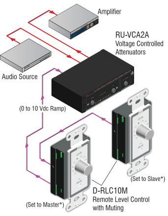
\* Each D-RLC10M may be set as Master or Slave on rear-panel switch; Master unit generates the 0 to 10 Vdc ramp.
