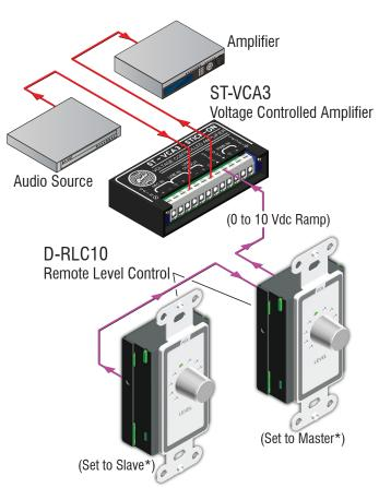
\* Each D-RLC10 may be set as Master or Slave on rear-panel switch; Master unit generates the 0 to 10 Vdc ramp.
