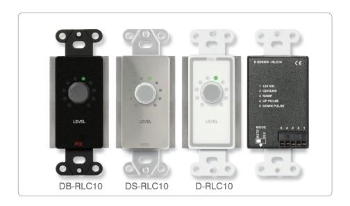
The D SERIES-RLC10 is a rotary remote level control that provides user adjustment at single or multiple locations. Optical encoder technology allows continuous knob rotation with a comfortable adjustment rate and long-term trouble-free and noise-free operation. These controls directly connect to any RDL VCA and OEM equipment with 0 to 10 Vdc ramp inputs.
